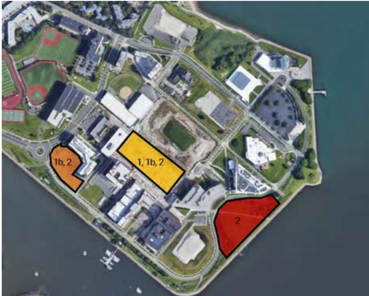
Figure 46: Possible geothermal field well locations
