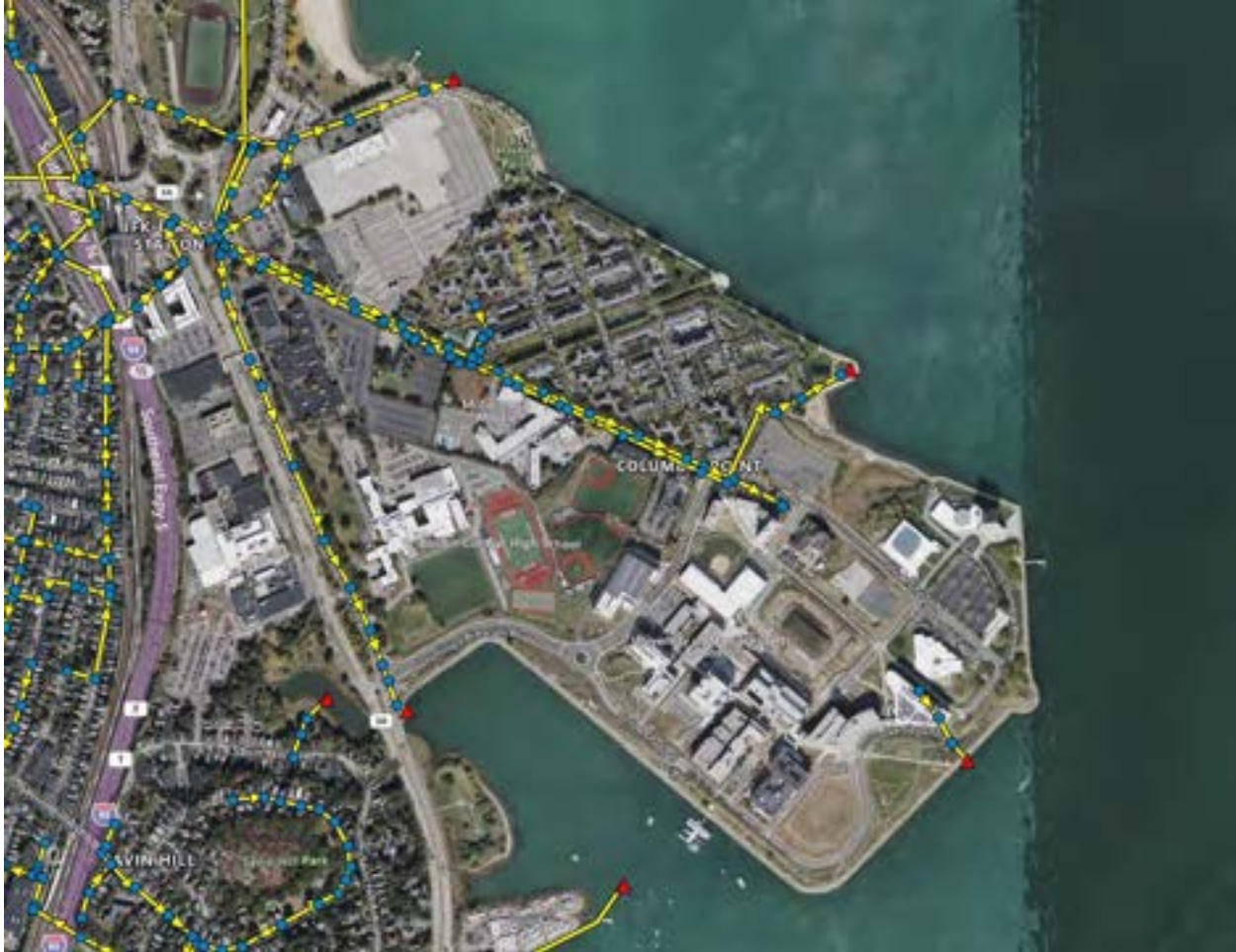
Figure 33: Boston Water and Sewer Commission inundation model indicating the locations of stormwater or wastewater pipes (yellow), manholes, catch basins, or pipe size changes (blue), and outfalls (red).
